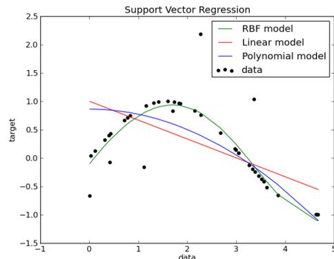
**Figure 5:** Support Vector Regression data-fitting with a rbf, linear, and polynomial kernel on a set of normally distributed data with random noise introduced into the data-set.
